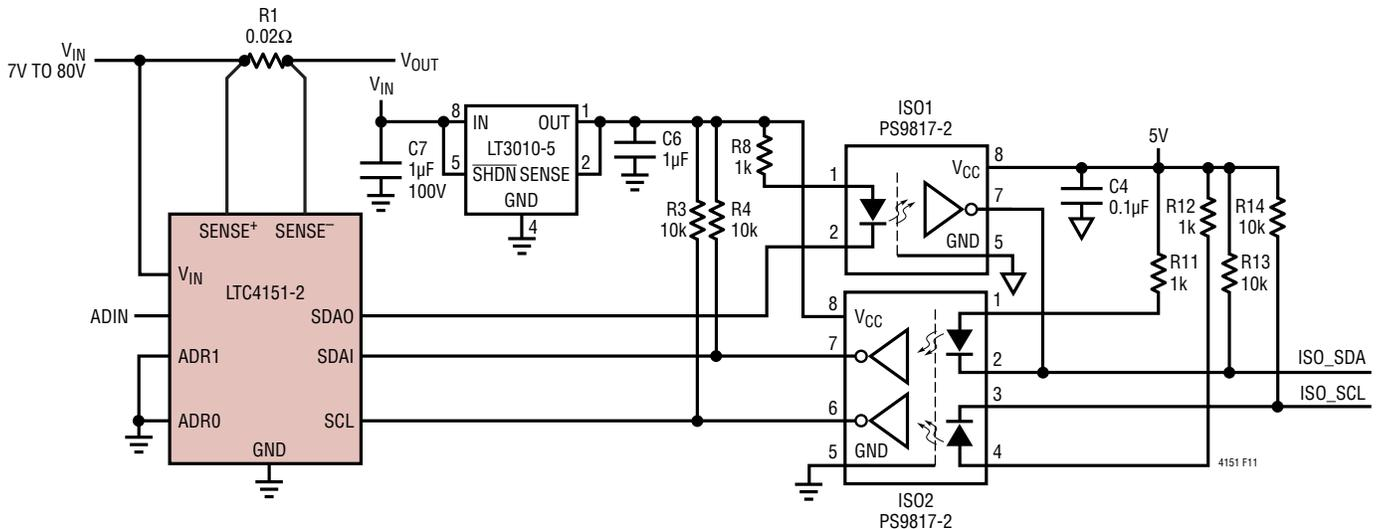
Figure 11. LTC4151-2 I<sup>2</sup>C Opto-Isolation Interface with High Speed Opto-Couplers
