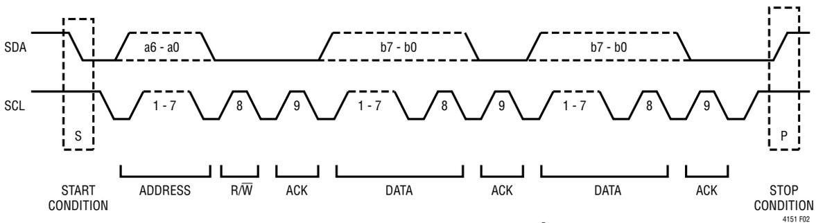
Figure 2. General Data Transfer over I<sup>2</sup>C
