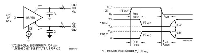
Figure 5. Driver Enable and Disable Timing Measurements
