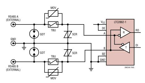
Network for IEC Level 4 Protection Against Surge, EFT and ESD Plus 360V Overvoltage Protection
