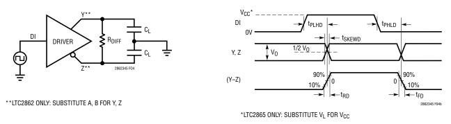
Figure 4. Driver Timing Measurement
