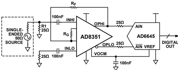
Figure 41. ADC Driving Application Using Single-Ended Input
