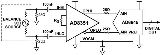
Figure 40. ADC Driving Application Using Differential Input
