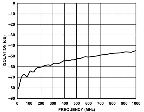
Figure 9. Isolation vs. Frequency ( $A_V = 10\text{ dB}$ )
