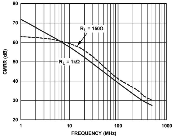
Figure 27. Common-Mode Rejection Ratio, CMRR ( $R_S = 100 \Omega$ )
