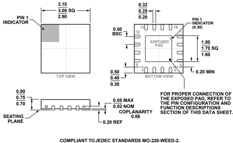
Figure 52. 16-Lead Lead Frame Chip Scale Package [LF CSP\_WQ]
