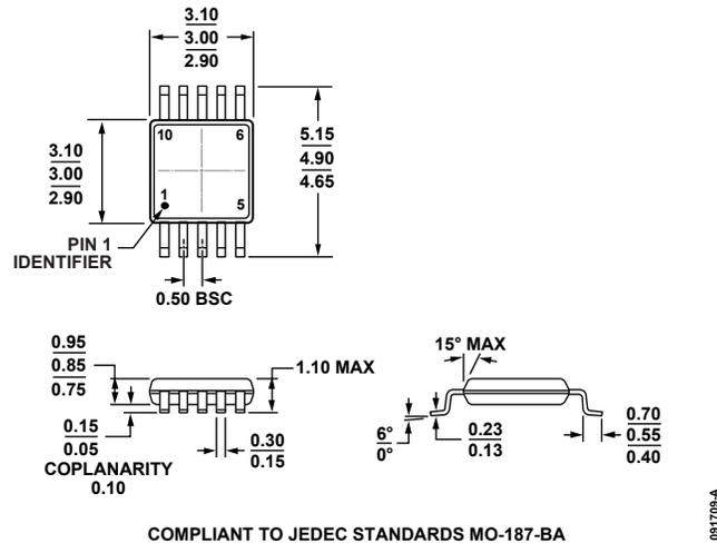
Figure 51. 10-Lead Mini Small Outline Package [MSOP] (RM-10)
