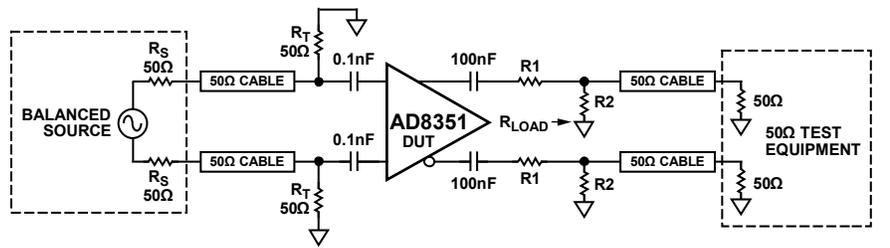
Figure 47. Test Circuit
